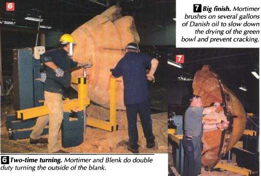
duty turning the outside of the blank.
