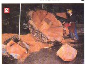
**2** Cutting away the waste. Mortimer removes excess wood from the inside and outside of the blank with a chainsaw, reducing the weight to around two tons. A center stem is left for attaching to the lathe's tailstock.
